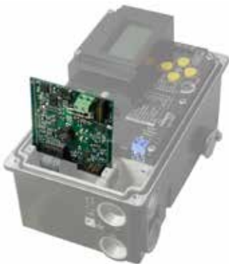
Auxiliary Card Being Installed
