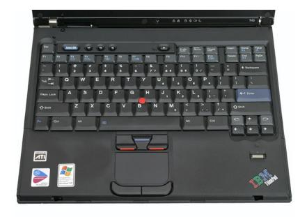
To the above left of the keyboard we have the blue Access IBM button, volume control buttons, and system power button just as they were laid out in earlier T4X notebooks. Future ThinkPads may not feature the Access IBM button, but a button simply labeled "Think" due to
