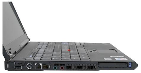
On the left we find the notebook lock, 2 USB 2.0 ports, 1 S-Video out port, 56kbps modem RJ11 port, 10/100/1000M Ethernet RJ45 port, earphone and microphone jacks, and CPU
