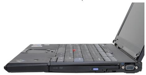
The T43 2668 44U we are testing has a 40GB HDD capacity. The Fujitsu-supplied HDD (model number MHT2040AH) spins at 5400rpm next to the 9.5mm HLDS 24X DVD/CDRW Combo drive.
