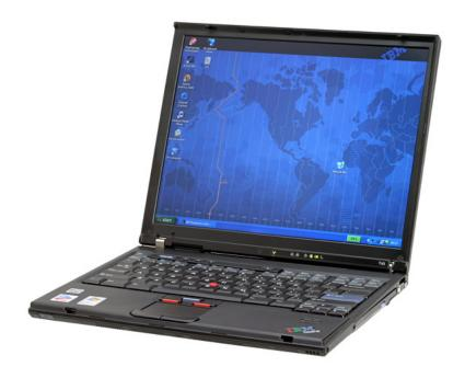
The T43 2668 44U equipped with 14.1" XGA resolution display. Like the T42, the T43 is also offered with 14.1" SXGA and 15.1" SXGA+/UXGA resolution display editions. Here are the specs for the T43 2668 44U:
