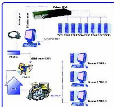
Prima IP as PPP client to dial-out to ISP for remote clients to access via internet
