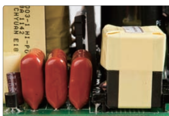
LLC Resonant Converter Topology achieves high efficiency
