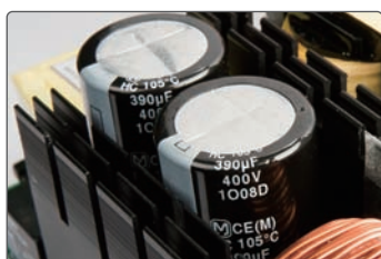
Solid State Capacitors and 100% 105°C Japanese Grade A Electrolytic Capacitors provide great reliability
