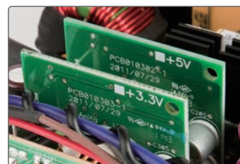
DC-to-DC Converter Design ensures system stability
