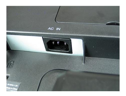
This is the monitor's AC in connector. As mentioned earlier, the QL-711V features an integrated inverter which is just what the office environment needs.
