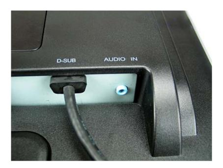
At the rear, the monitor is equipped with the analog D-Sub connector and an audio-in port for the speakers.
