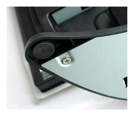
While the base stand has limited features, the detail and workmanship are very good. With the monitor stood on its side, we discover three rubber "feet" to provide more friction that will stop the monitor from moving unnecessarily.
