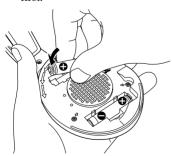
Be sure to use the supplied exclusive battery. Do not use any other rechargeable or dry cell battery, which may cause malfunctions or damage the unit.
