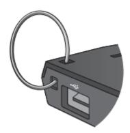
**Note:** Security cable loop is not included. You can build one – insert a length of quality wire rope (<3mm) through the security opening and then crimp the ends together with a cable sleeve.
