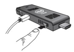
If the Intel Compute Stick is plugged into the HDMI port of a TV or display that also has a USB port, there MAY be enough power on the USB port to power it. To do this, plug the micro-USB end of the 3-foot USB cable into the Intel Compute Stick and the standard USB end of the cable into the USB port on the TV (instead of using the AC power plug).
