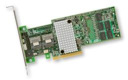
help protect data stored in the controller cache. The benefits of this technology are elimination of hardware maintenance associated with LiON batteries, lower total cost of ownership over the life of the adapter, and more environmentally friendly cache protection.
