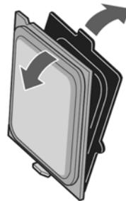
**Figure 15. Remove Processor Protective Cover**
