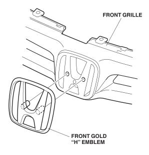
5. Slide the push nuts onto the pins. Note the direction of the push nuts.
