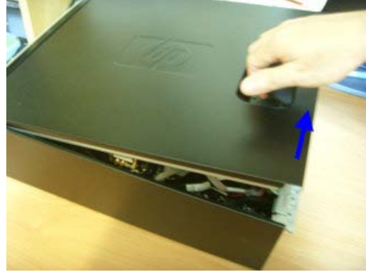
Figure 2: Rise access panel Press front panel clip
