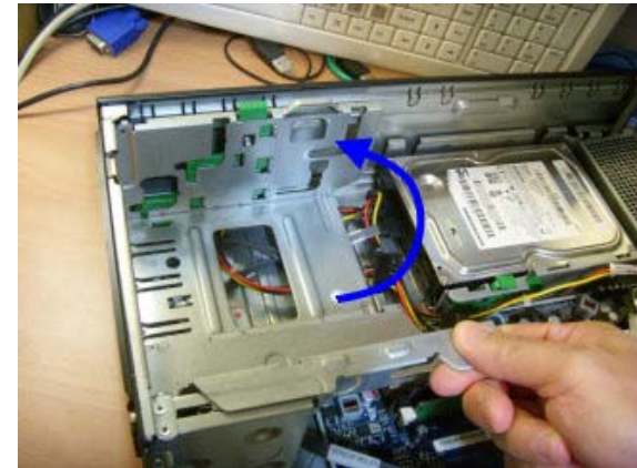
Figure 18: Rotate ODD cable to vertical
