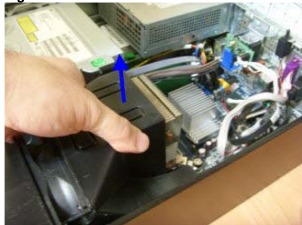
Figure 6: Release Fan duct
