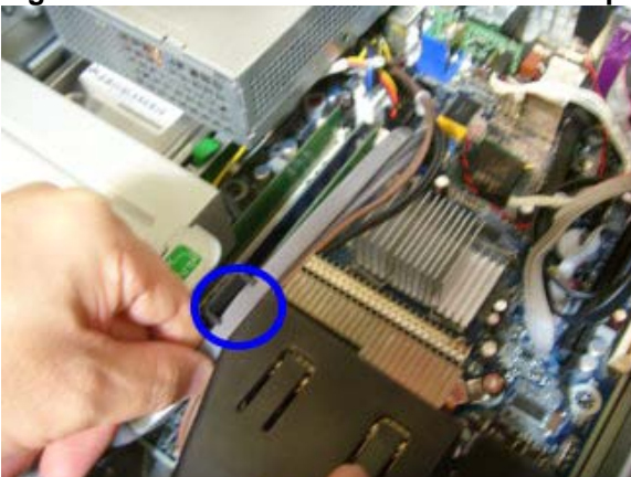
Figure 5: Remove all cable from cable clamp
