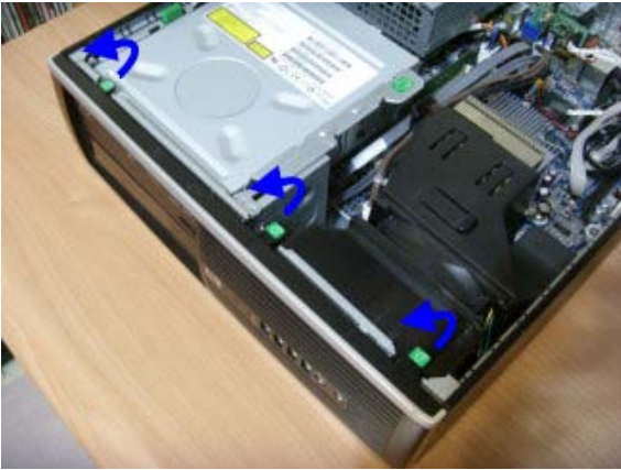
Figure 5: Remove all cable from cable clamp
