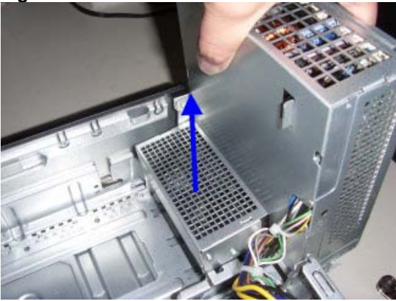
Figure 21: Remove PSU from Chassis
