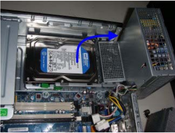
Figure 21: Remove PSU from Chassis
