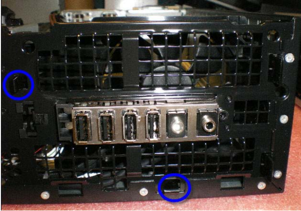
Figure 7: Press 2 clip to Remove Fan holder from front chassis,
