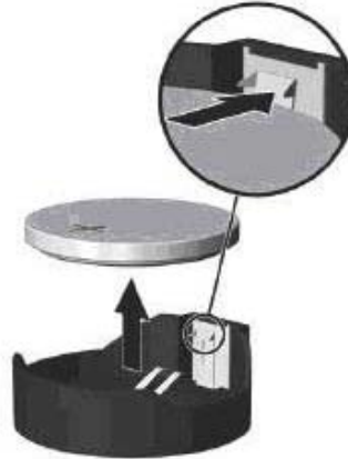
Figure 24: Press Battery holder and Pull battery
