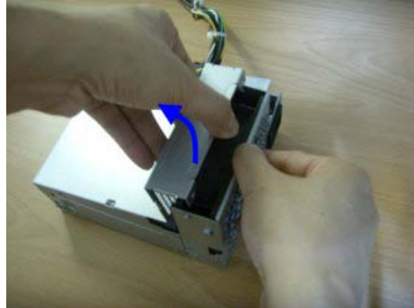
Figure 28: Remove PSU the top of case
