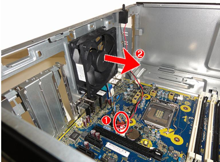
To install the fan assembly, reverse the removal procedure. Be sure to orient the air flow out of the unit.
