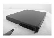
Mount the ears to the front side of the enclosure by securing the ears to the side of the enclosure with the included screws.
