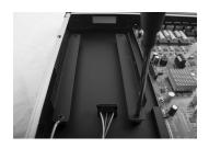
Remove the two drive trays from the enclosure by removing the screws at the base of the bracket.
