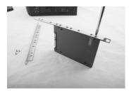
Mount the 2.5" drive between the two trays with the four screws in the plastic screw package.
