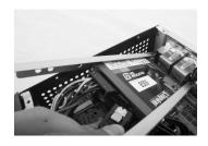
Connect the SATA cable to the complete HDD
