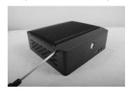
Using a phillips head screw driver, remove the four screws on the sides of the enclosure.
