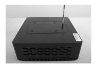
Using a phillips head screw driver, remove the three screws on the bottom cover.
