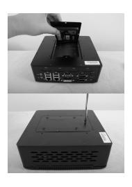
Make sure the HDD port in the right position, and then connect the 2.5" HDD head to the HDD port.
