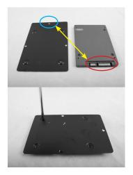
In order to connect the 2.5" HDD to the HDD port correctly in the next step, make sure the HDD head is on the opposite side of the top mounting screw hole.
