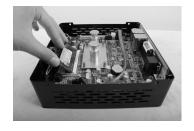
Align notch in memory circuit with corresponding guide on the memory slot. Insert the memory circut at a 45° angle and press the circuit flat and secure it to the memory slot with an audible click on each side of the memory slot.
