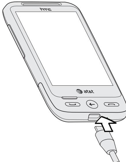
3. Plug in the power adapter to an electrical outlet to start charging the battery.
