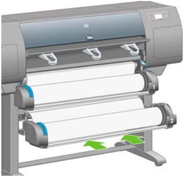
14. Using the stops at each end of the spindle, carefully wind the excess paper back onto the spindle.
