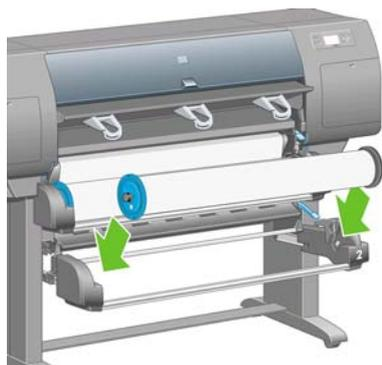
9. Lift the drawer 2 paper load lever. This is located on the right-hand side of the printer and under drawer 1.
