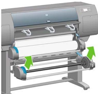
7. Load the spindle using the same procedure as already described for roll 1.
