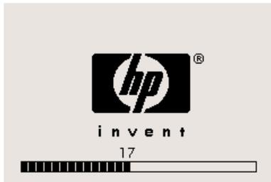
If the printer's start-up process stops when the front panel is displaying the number 17, this indicates that there is a problem with the file system on the printer's hard disk, so the printer is checking the whole file system and making any necessary corrections. This problem can arise when there has been a power cut while the printer was switched on, or if there is a physical problem with the hard disk.
