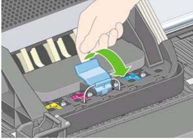
5. Lift up the cover. This will give you access to the setup printheads.
