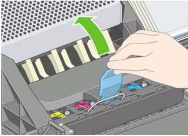
6. Before removing the setup printheads, look at the window on top of each one and check that the printhead contains ink.
