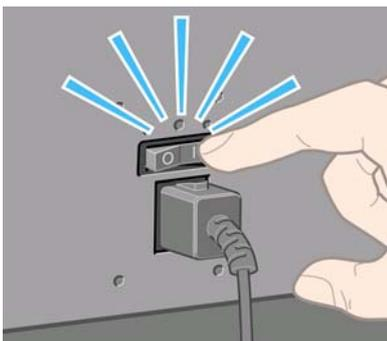
7. If the power light on the front panel remains off, press the Power key to switch on the printer.
