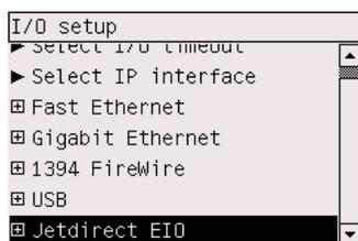
The front panel will reveal whether the print server is **Installed** or **Not installed**.
