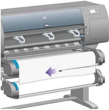
5. Remove the cut-off piece of paper.
