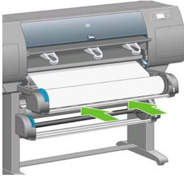
21. Using the stops at each end of the spindle, carefully wind the excess paper back onto the spindle.
