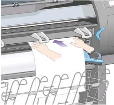
7. Insert the sheet until it reappears from the printer as shown below.
