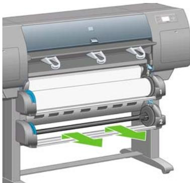
6. Remove the spindle from drawer 2.
