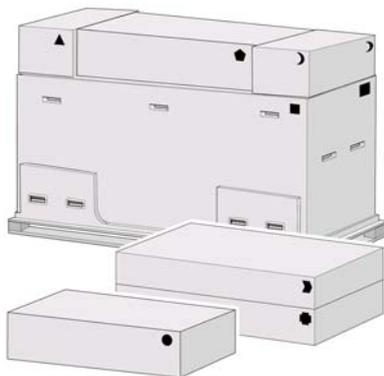
4. Remove the two lids. Place the consumables and spare boxes in front of the printer body. Lower the stand and bin box onto the consumables and spare boxes. Then lower it onto the floor.
