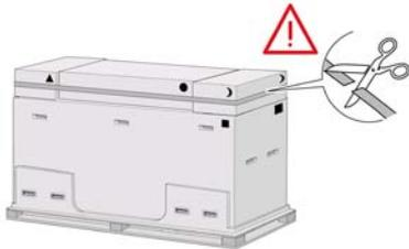
3. Remove the boxes from the top of the main printer box.
