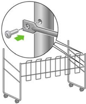
5. Attach the second cross frame to the bin assembly using four screws.
