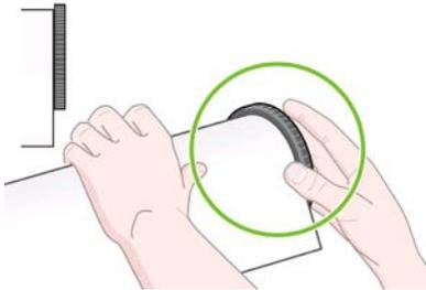
7. Put the blue paper stop on to the other end of the spindle, and push it towards the end of the roll.
