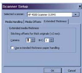
5. Change the value for each of the scanner's cameras. Normally, only positive values should be used.
