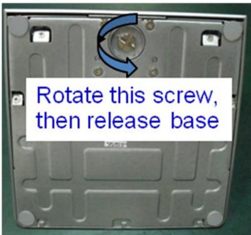
Step 2: Strip the screws from rear cover so that the rear metal cover can be removed , after be turn back;
