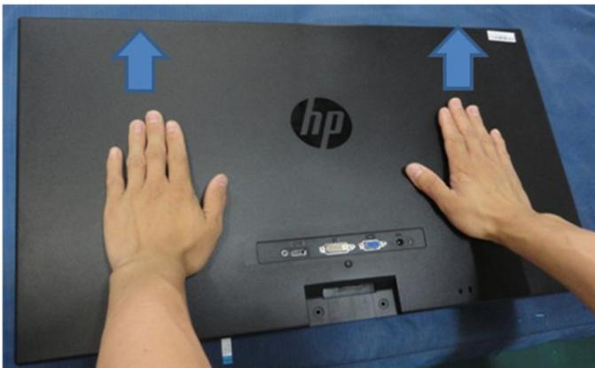
Step 4: Push up and disassemble the cover from the panel;
