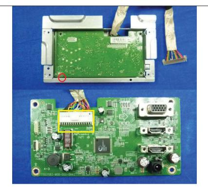
Remove the screws and disconnect the connectors to remove the MAIN BOARD
