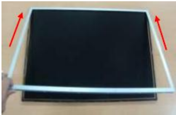
3.Separate C/Top ( push the C/Top because of damages on COF)
