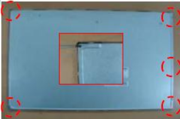
5. Loosen B/L Screw (*5)
