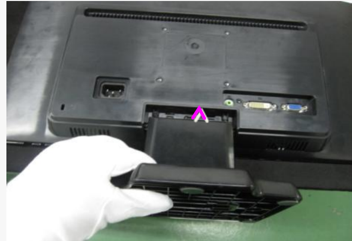
2. Demount Stand & Remove Stand Base Form Display.
