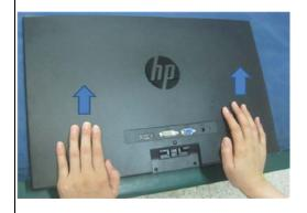
Step 5: To remove the shielding(contain the other material);
