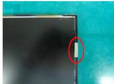
Step5 : Detach AL tape on board ass'y
