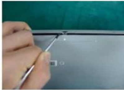
Step2 : Dismantle the case top (down)
