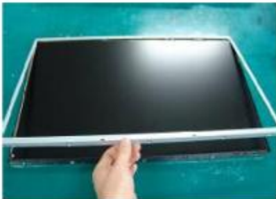
Step4 : Separate case top (push the case top because of damages on COF)
