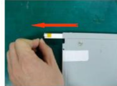
Step9 : Pull lamp housing with hands normal to LCM (*Be careful not to break the Lamp)
