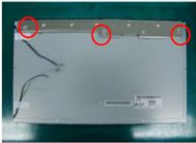
Step1 : Unfix the Screw (3 Point) Remove the cover shield
