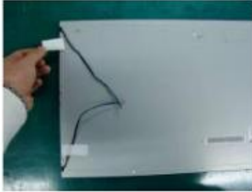
Step7 : Separate wires from the tape (2 Point)
