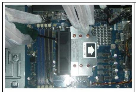
7 Remove CPU cooler from PCA
