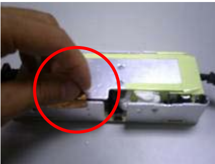
FIGURE 19: Removing the sheet metal shielding: Remove two screws
