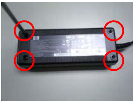
FIGURE 12: Removing the power supply covers
