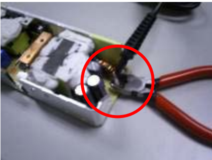
FIGURE 23: Removing the white thermal paste
