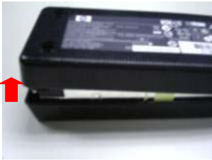
FIGURE 14: Removing the power supply bottom cover
