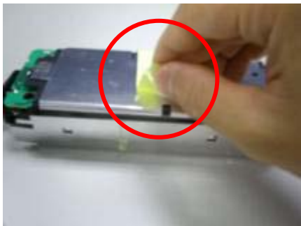
FIGURE 16: Removing the bottom aluminum shielding
