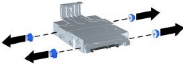
FIGURE 5: Removing the guide screws
