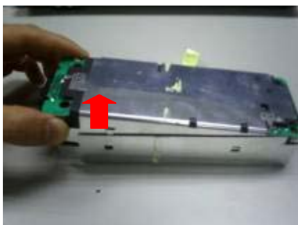
FIGURE 16: Removing the bottom aluminum shielding
