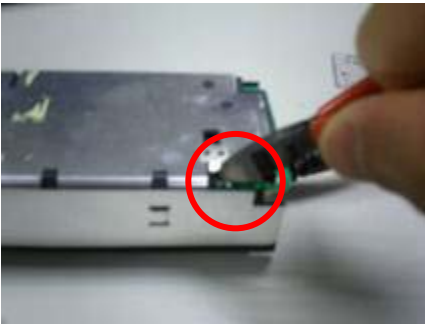
FIGURE 18: Removing the sheet metal shielding: Tear foil
