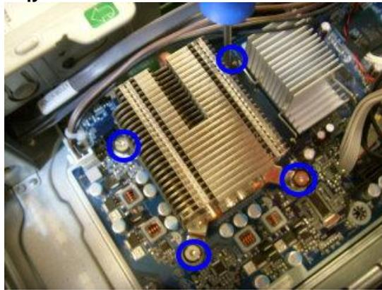
**Figure 11: Remove Heat sink from PCA**
