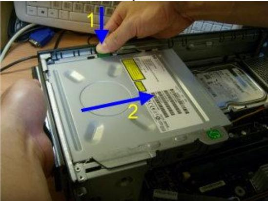
**Figure 18: Rotate ODD cable to vertical**
