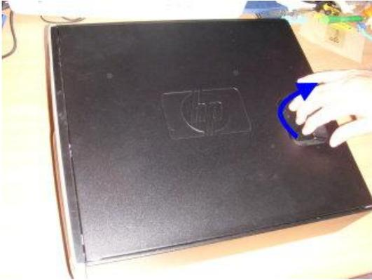
**Figure 2: Rise access panel Press front panel clip**
