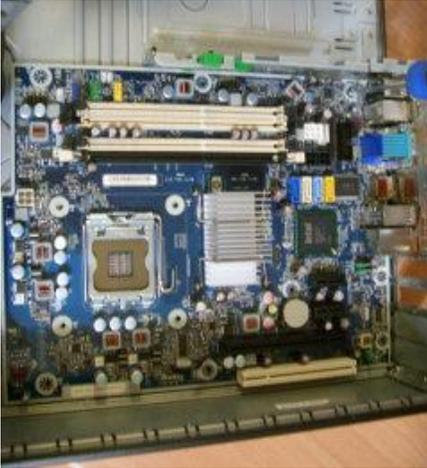
**Figure 16: Remove all internal cable from PCA**
