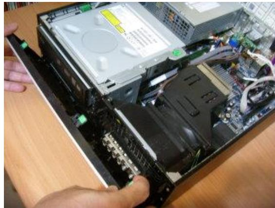
**Figure 5: Remove all cable from cable clamp**
