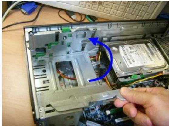
**Figure 19: Rotate PSU to Vertical**
