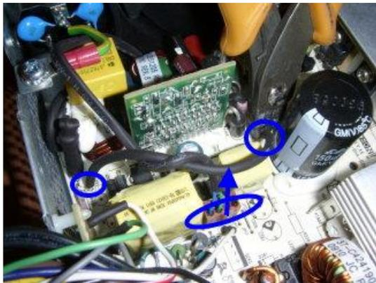
**Figure 30: Remove PSU PCS 5 screws**
