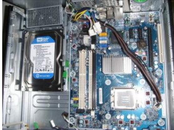
**Figure 17: Release ODD from ODD cage
