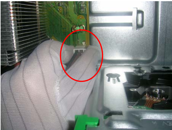
Figure 7: Disconnect the cables from the board
