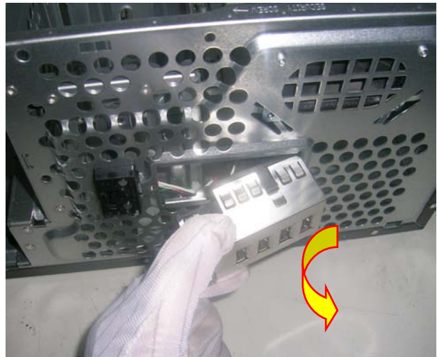
Figure 32: Rotate the Front I/O and pull it out of the chassis
