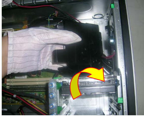
Figure 12: Loosen the clip that secures the heat sink to the system board.
