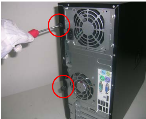
Figure 1: Remove the two screws
