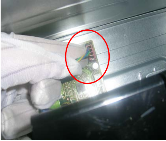
Figure 7: Disconnect the cables from the board
