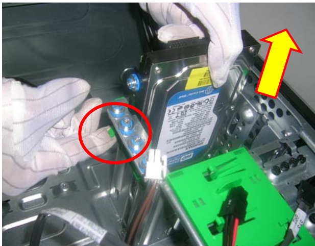
Figure 19 : Pull the handle and lift the HDD off the unit
