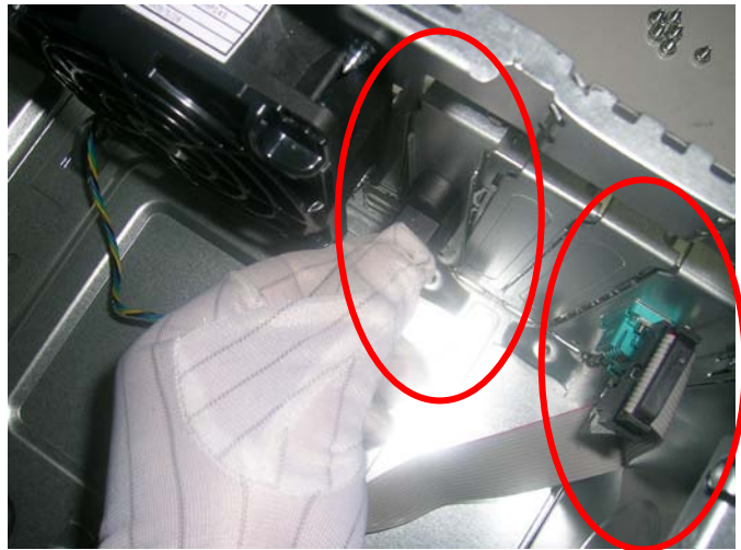
Figure 28: Remove the shielding
