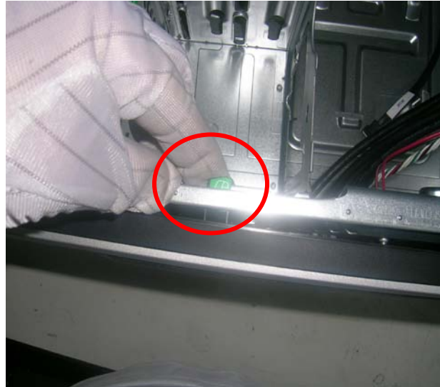
Figure 24: Rotate the bezel off the chassis
