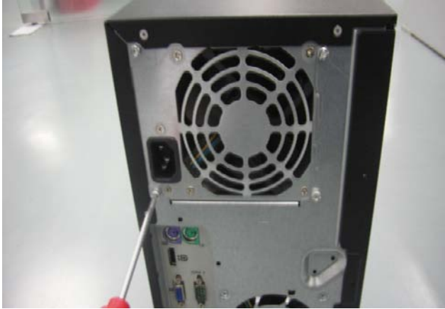
Figure 9 Loose the screws from system fan
