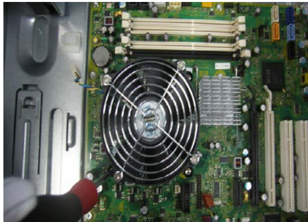
Figure 12 Loose the screws and remove CPU fan
