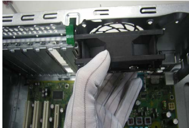
Figure 12 Loose the screws and remove CPU fan
