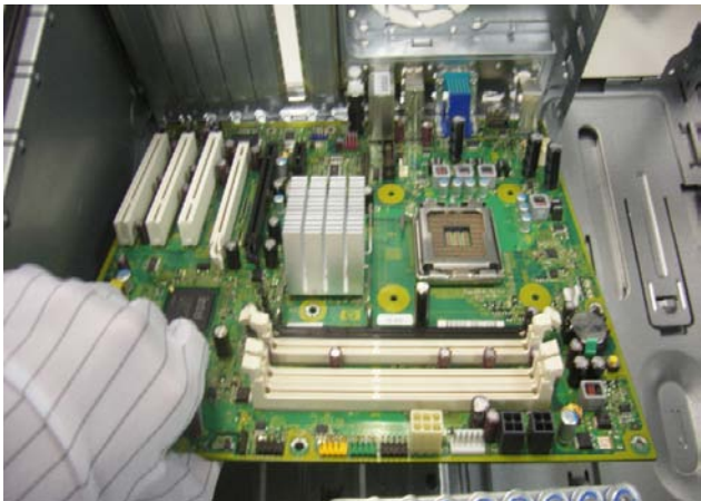
Figure 17 Remove M/B from chassis
