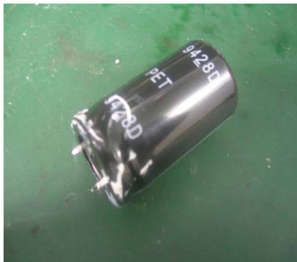
Figure 26 Remove the Electrolytic Capacitors
