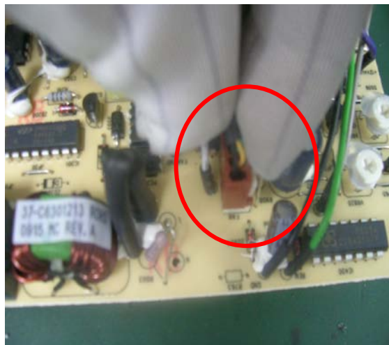
Figure 24 Remove the power supply PCA from the power supply chassis
