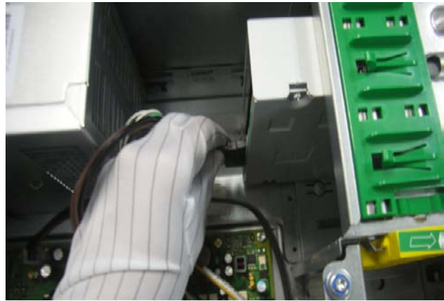
Figure 4 Disconnect the cables from the ODD
