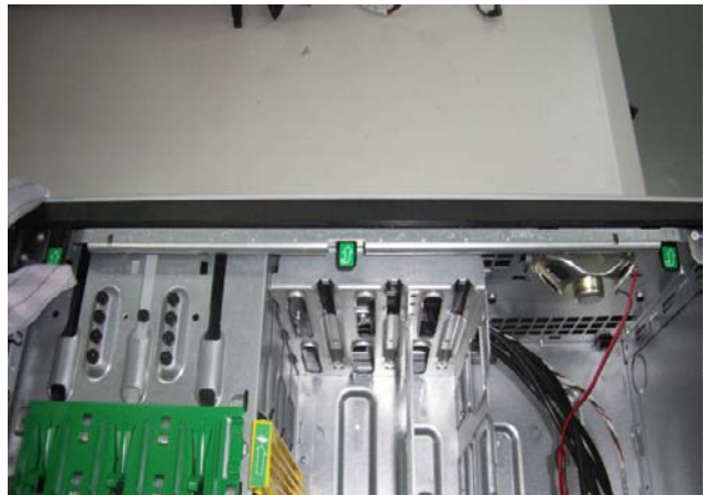
Figure 18 Remove front panel
