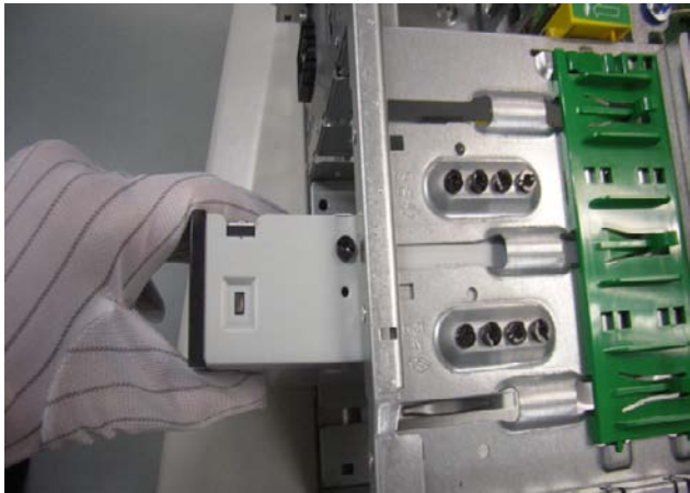
Figure 21 Lift the cover off the power supply
