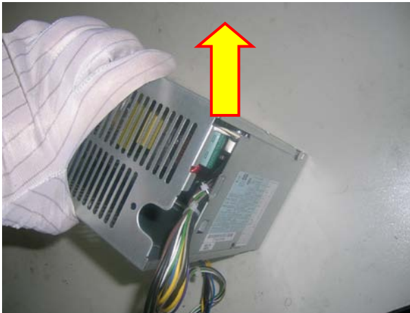
Figure 21 Lift the cover off the power supply
