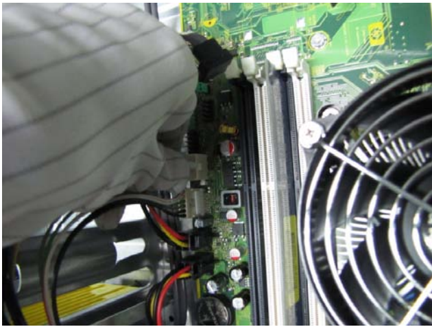
Figure 3 Disconnect PSU cables from the board
