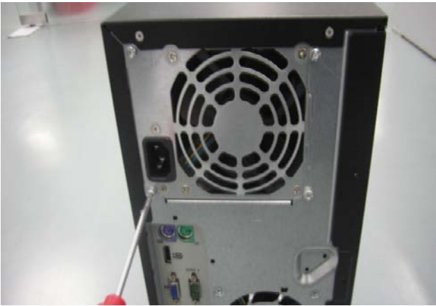
Figure 9 Loose the screws from system fan
