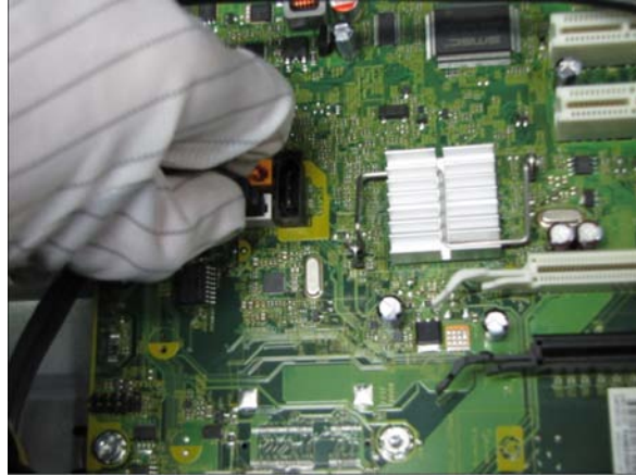
Figure 2 Disconnect the cables from the board
