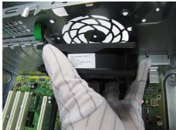
Figure 10 Remove system fan
