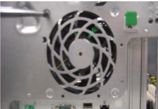
Figure 9 Loose the screws from system fan
