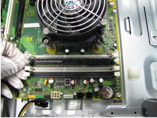
Figure 13 Rotate the handle and open it up
