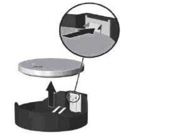
Figure 15 Remove the battery from the system board
