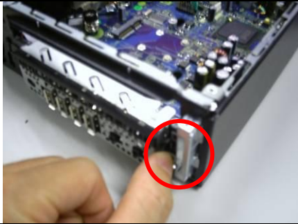
a) Press snap to unfix I/O cage
