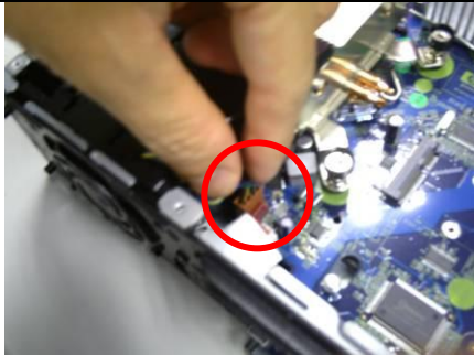
a) Disconnect fan cable by hand
