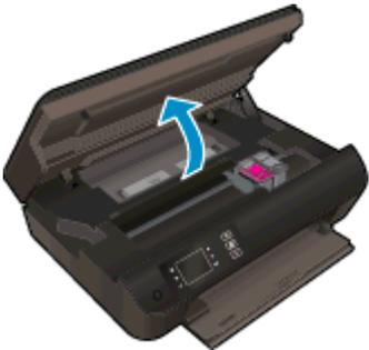
2. Remove the jammed paper from inside the printer.
