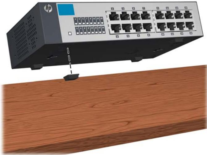
Figure 2-8. Horizontal surface mounting
