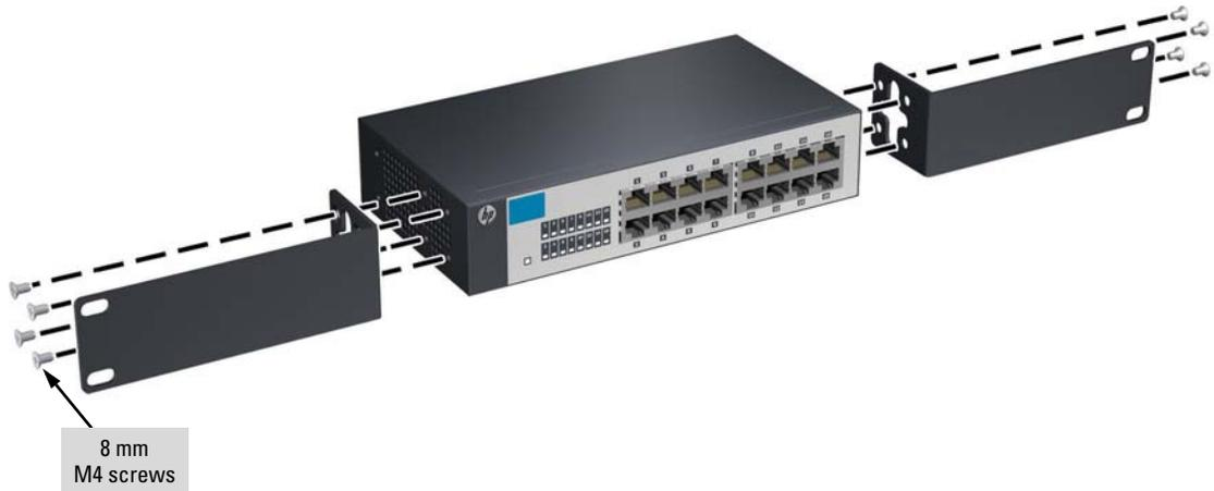
**Figure 2-3. Attaching mounting brackets to the V1410-16 Switch**
