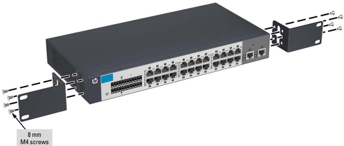
**Figure 2-4. Attaching mounting brackets to the V1410-24 and V1410-24-2G Switch**
