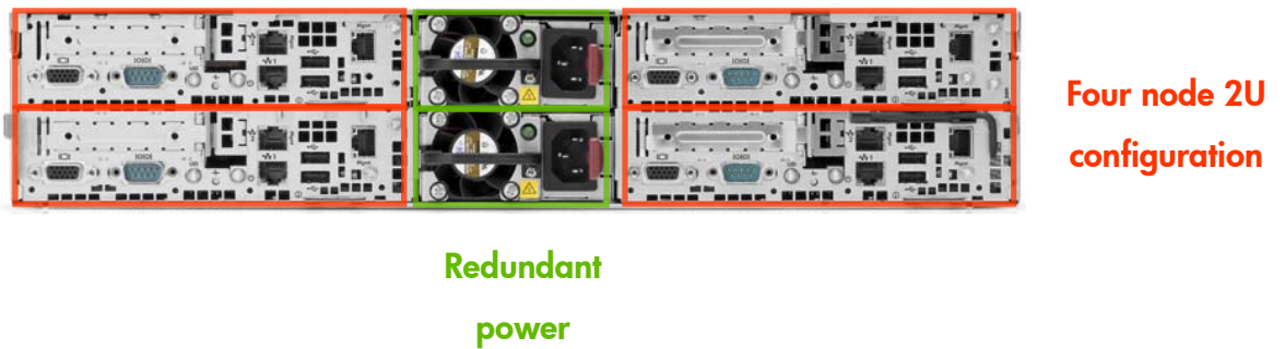
Figure 8. DL1000 four node configuration – rear chassis view
