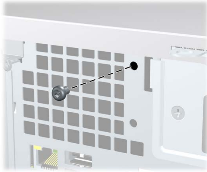
Figure 2-1 Removing the Smart Cover Lock Screw
