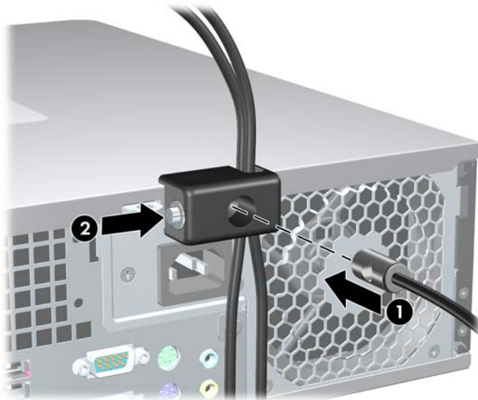
Figure C-6 Engaging the Lock
