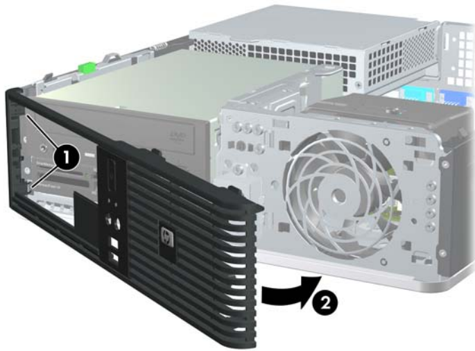
Figure 2-7 Replacing the Front Bezel
