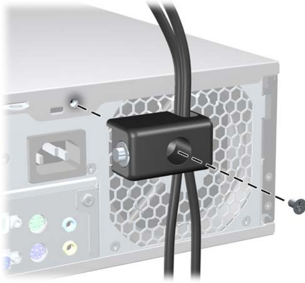
Figure C-5 Attaching the Lock to the Chassis
