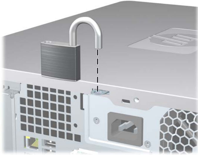
Figure C-2 Installing a Padlock
