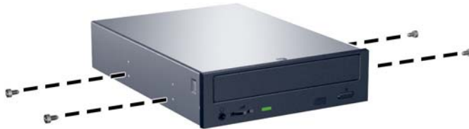
Figure 2-27 Installing Guide Screws in the Optical Drive
