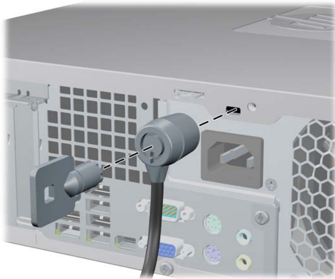
Figure C-1 Installing a Cable Lock
