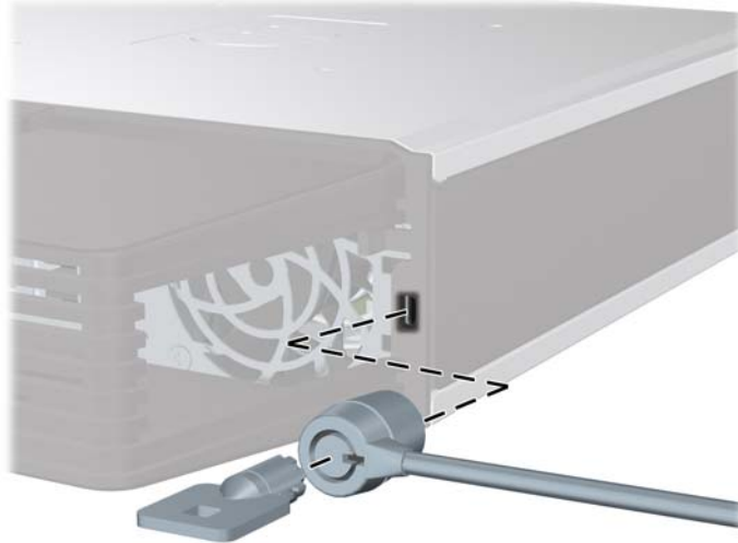
Figure C-2 Installing a Cable with a Port Cover Installed
