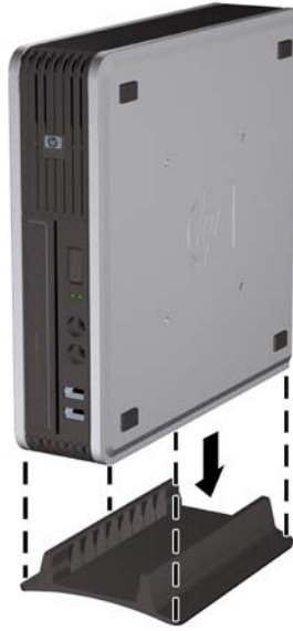
Figure 2-9 Placing the Computer on the Stand
