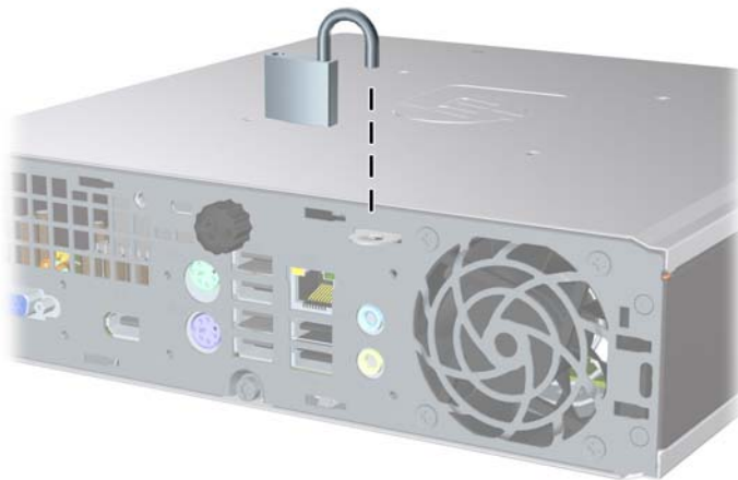
Figure C-3 Installing a Padlock
