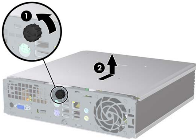
Figure 2-2 Removing the Computer Access Panel
