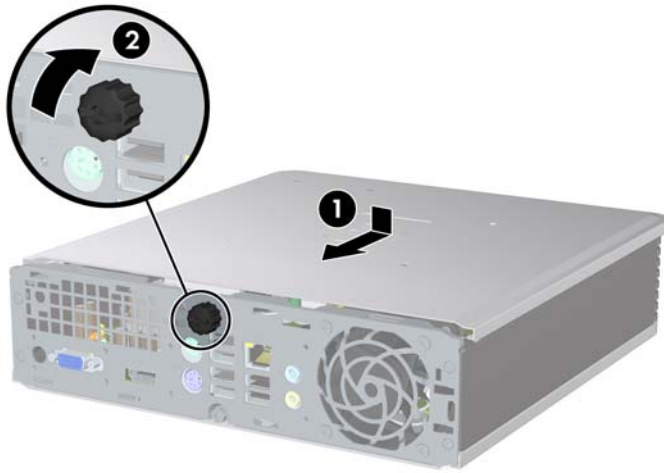
Figure 2-3 Replacing the Computer Access Panel
