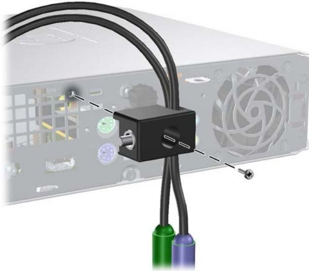
Figure C-6 Attaching the Lock to the Chassis
