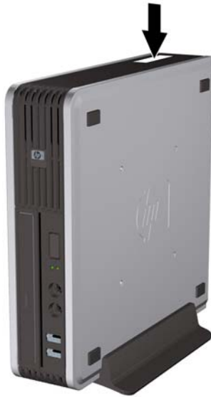
Figure 1-5 Serial Number and Product ID Location
