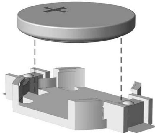
**Figure 3-1** Removing a Coin Cell Battery (Type 1)
