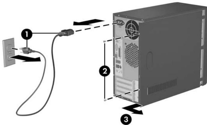
**Figure 2-1** Removing the Power Cord and Access Panel
