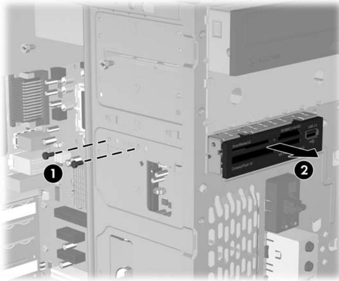
**Figure 2-11** Removing a 3.5" Device (Media Card Reader Shown)
