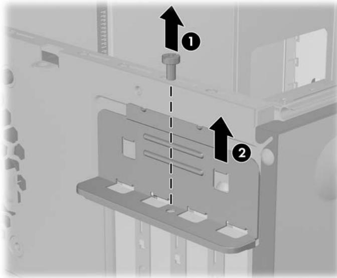
**Figure 2-6** Releasing the Slot Cover Lock
