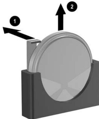
**Figure 3-3** Removing a Coin Cell Battery (Type 3)
