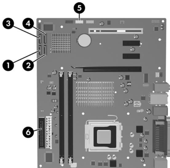
**Figure 2-9** System Board Drive Connections
