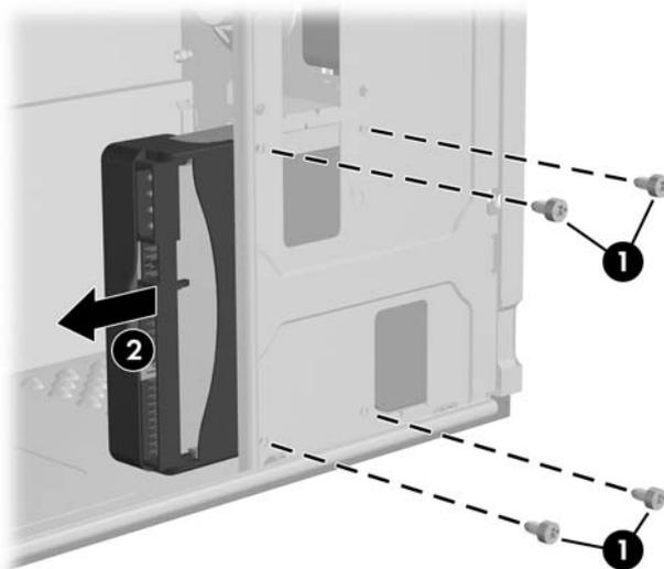
**Figure 2-12** Removing a 3.5" Hard Drive
