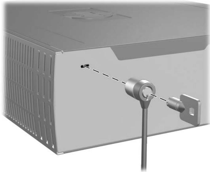
**Figure 2-13** Installing a Security Lock
