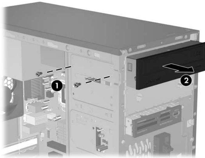
**Figure 2-10** Removing a 5.25" External Drive
