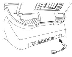
3) Plug the AC cable into the outlet.
