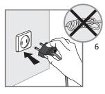
**5-6** Place the thermostat in the minimum position before plugging in the appliance.
