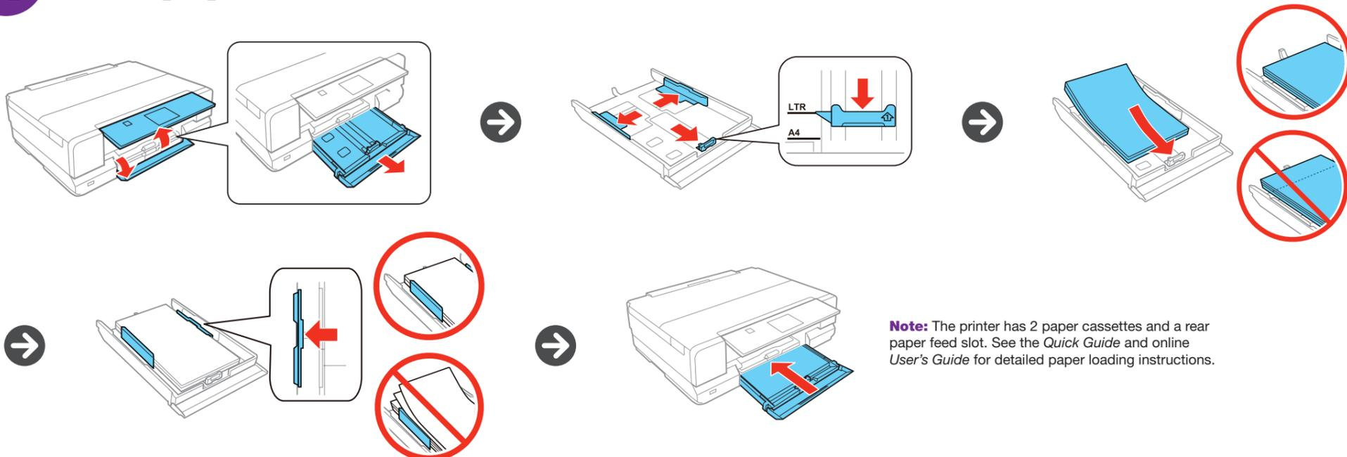
**Note:** The printer has 2 paper cassettes and a rear paper feed slot. See the *Quick Guide* and online *User's Guide* for detailed paper loading instructions.
