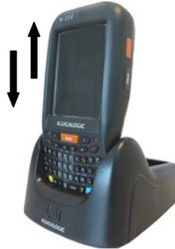
Figure 2 - Mobile Computer Insertion
