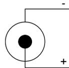
Figure 3 - Power Supply Polarity
