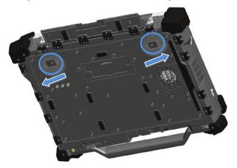
4. Use the tab on the bottom of the battery to remove the battery from the computer.
