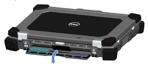
3. Press outward on the two battery release latches on the bottom of the computer.
