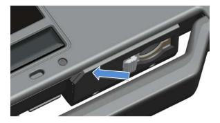
The Secure Digital card can be fully inserted, allowing the protective door to be closed. Insert the card into the secure digital slot until it is fully seated in its connector. To release the secure digital card, press in on the card edge and the reader will eject the card.
