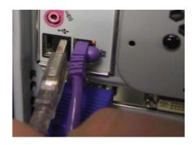
Attach an Ethernet cable to the Ethernet port on the DUB-E100.
