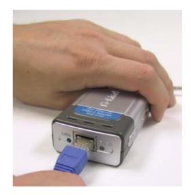
Attach the other end of the Ethernet cable to your network switch, hub, or router.
