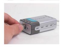
Attach the other end of the CAT5 Ethernet cable to a switch, hub, or router/gateway.
