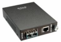
DMC-810SC Media Converter: This converter converts 1000BASE-T Gigabit twisted-pair signals to 1000BASE-LX Gigabit single-mode fiber signals. Maximum fiber cable distance is 10km. 1 RJ-45 port and 1 fiber port (SC type connector) are provided.
