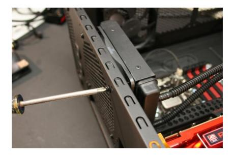
Select the fan mounting point on your specific case. Insert the 4 fan screws through case and through the 4 holes on the H50 fan. Then, insert the 4 screws into the corresponding holes on the H50 radiator and tighten the screws evenly.
