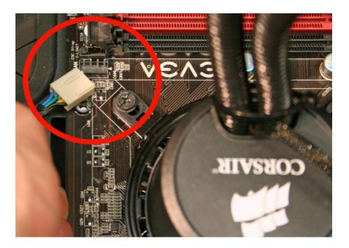
Connect the fan and pump connectors to available headers on your motherboard. Now, your installation is complete!
