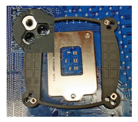
Install the back plate onto the motherboard using the adhesive tape. Be sure to orient the plate correctly for the CPU you are using.
