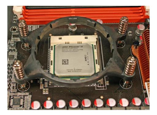
The attachment method is the same for AMD processors as it is for Intel processors.
