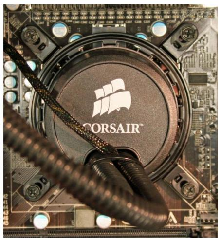
Tighten the screws in an "X" pattern to distribute the pressure evenly across the CPU.
