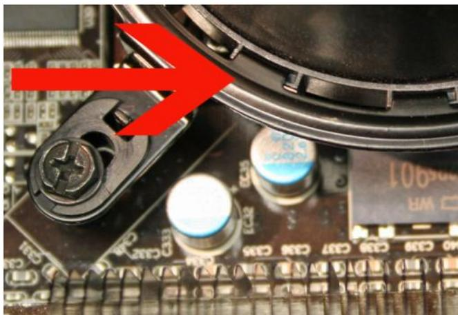
Twist the cooler to align the tabs on the bracket into the grooves on the cooler
