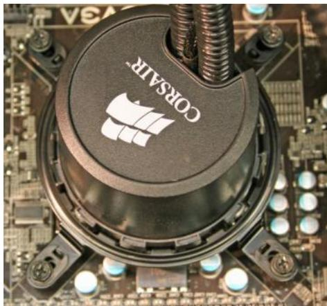
Align the 4 screws from the locking ring with the 4 mounting holes of the back plate. Tighten each screw only 1-2 turns, leaving room to move the cooler. Apply the cooler to the CPU.
