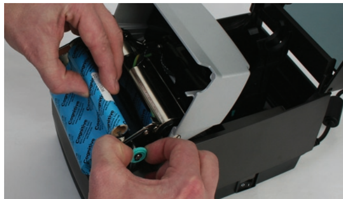
Figure 2-33. Pulling the Take Up Spindle Out to Insert Take Up Roll
