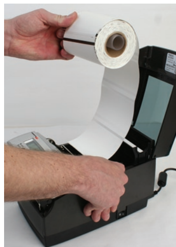
Figure 2-43a. Media Print Side Must be Facing Up for Inward Wound Media
