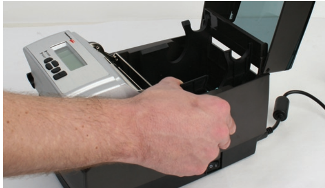
Figure 2-56. Opening the Media Guides
