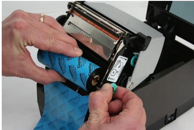
Figure 2-27. Lining up Ribbon Supply Core Notches with Supply Spindle Notches
