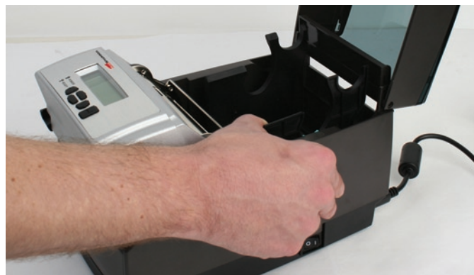
Figure 2-41. Spread the media guides apart
