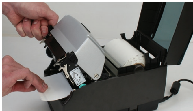
Figure 2-49. Pulling the Media Three to Four Inches then Centering on the Platen
