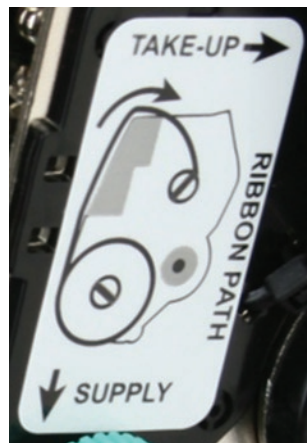
Figure 2-19: Ribbon Loading Label
