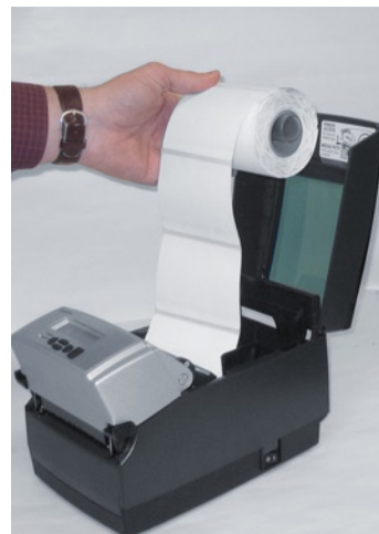
Figure 2-43b. Media Print Side Must be Facing Up for Outward Wound Media
