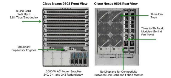
Figure 1. Cisco Nexus 9508 Switch
