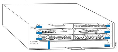
Figure 4 Tamper Evidence Label Placement (Front View)
