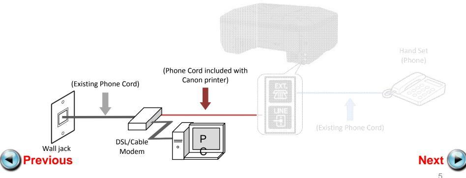
Plug the provided phone cord into the "LINE" jack on the rear of the multifunction.
