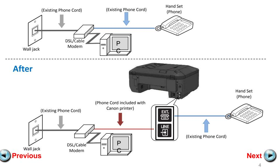
Plug the provided phone cord into the DSL/Cable Modem.
